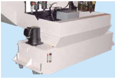
Coolant unit (tank)
